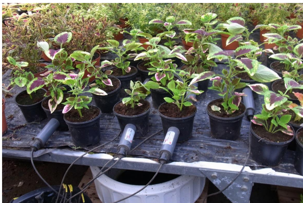
Figure 1 Soil moisture sensors installed at a commercial nursery to understand how manual irrigation of potted Coleus ( Solenostemon ) affects soil moisture
